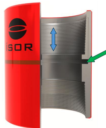
Figure 6. The Flexible Coupling (FC) enables thermal expansion of casing joints where the allowed movement (blue arrow) closes the thermal gap (green arrow) within the FC, limiting thermal stresses in the casing.
