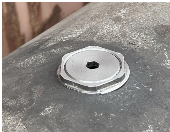
Figure 9. A prototype of the APB-Casing Collapse Protector fitted into a 13-3/8" casing.
