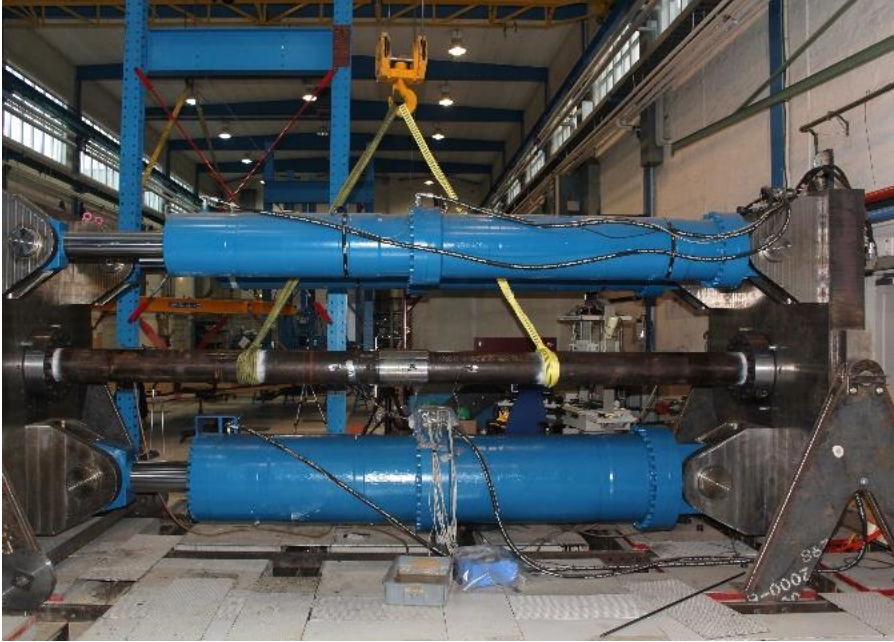
Figure 8: Flexible Coupling prototype testing at ambient temperature at SINTEF, Norway.
