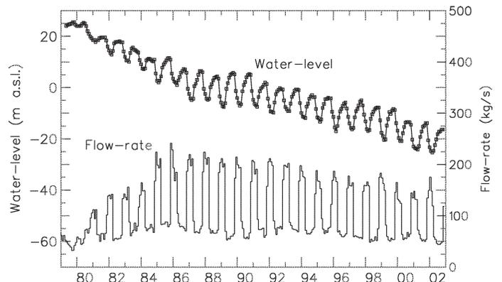
**Figure 6.** Production and water level history of the Beijing Urban sedimentary low-temperature geothermal system in China from 1979 to 2002. Based on Liu et al. (2002).
