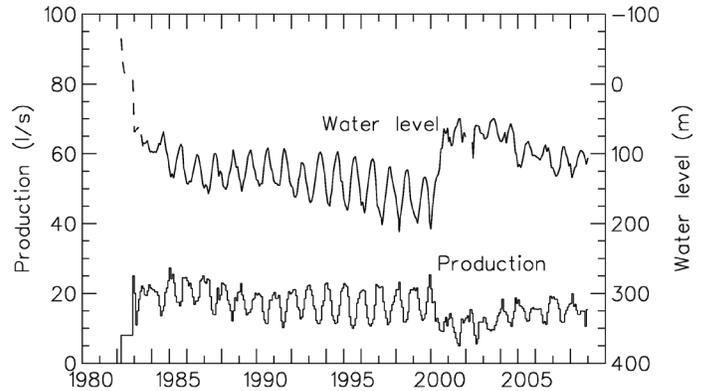
**Figure 4.** Production and water level history of the Gata low-temperature geothermal system in the Holt district of southern Iceland from 1982 to 2008. The broken line indicates estimated water level. From Axelsson et al. (2010b).
