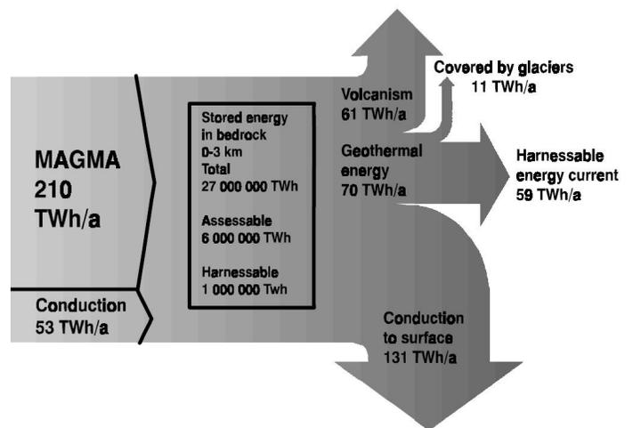
Figure 1. Simplified sketch of the geothermal resources of Iceland, reflecting their double nature. Based on combining an assessment of the terrestrial energy current in Iceland and an assessment of the heat stored in the crust (Stefánsson, 2000).
