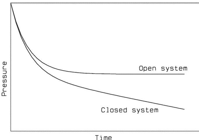
**Figure 2.** Schematic comparison of pressure decline in open (with recharge) or closed (with limited or no recharge) geothermal systems at a constant rate of production (from Axelsson, 2008a).
