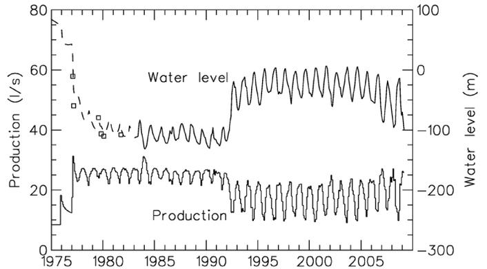
**Figure 5.** Production and water level history of the Skútudalur low-temperature geothermal system in Siglufjörður, N-Iceland, from 1975 to 2008. The broken line indicates estimated water level and the boxes isolated water level readings. From Axelsson et al. (2010b).
