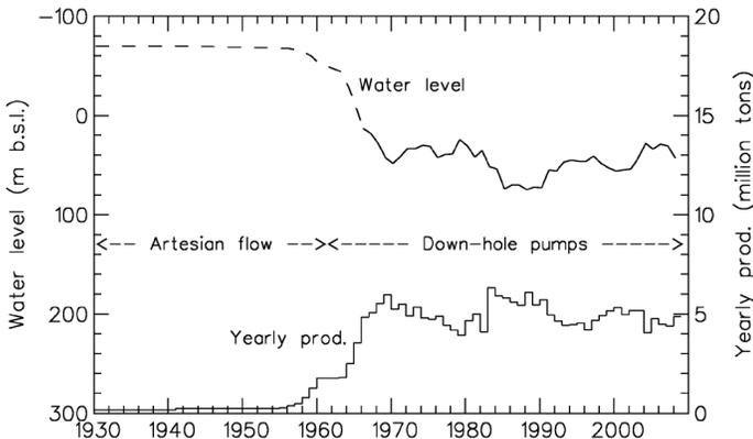
**Figure 3.** Production and water level (winter minima) history of the Laugarnes low-temperature geothermal system within Reykjavík, SW-Iceland, from 1930 to 2008. The broken line indicates estimated water level. From Axelsson et al. (2010b).
